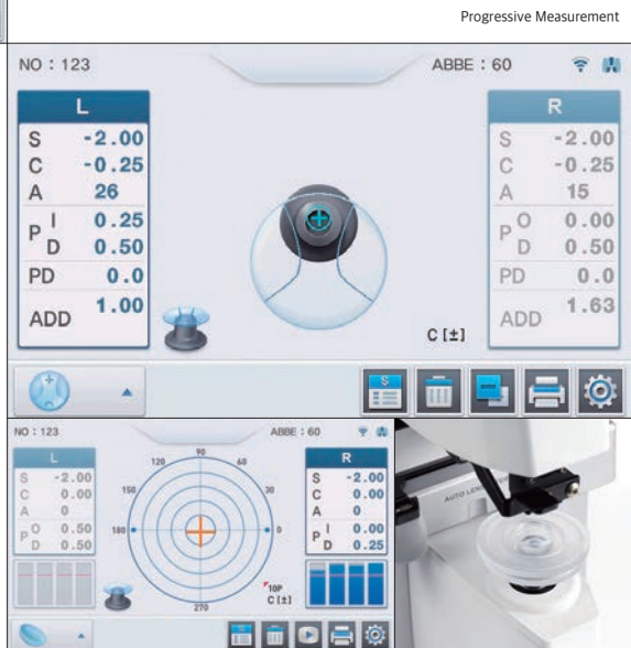
Contact Lens Measurement
